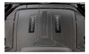
Carbon Fibre Engine Cover
